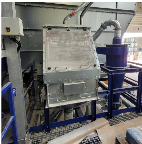
Figure 2: Sorbent dosing station feeding into the storage hopper
