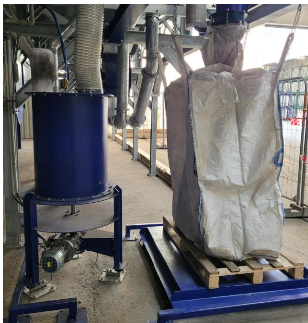
Figure 3: Sorbent storage hopper with sorbent dosing, placed on strain gauges.
